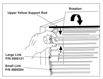
Figure 8. Removing Conveyor Belt
